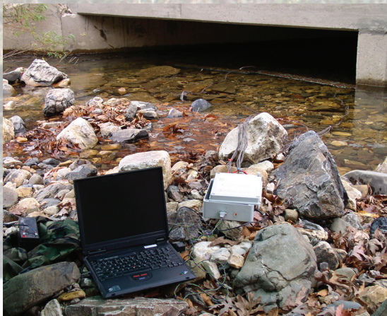
The device consists of a weatherproof control box connected to a series of sensor pads. The computer is only required for initial setup.
